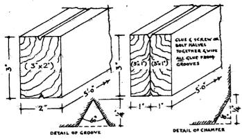
ALTERNATIVE CONSTRUCTION FOR ONE OR TWO PIECE VBLOCK
