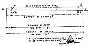
METHOD OF TAPERING GROOVE IN V BLOCK
