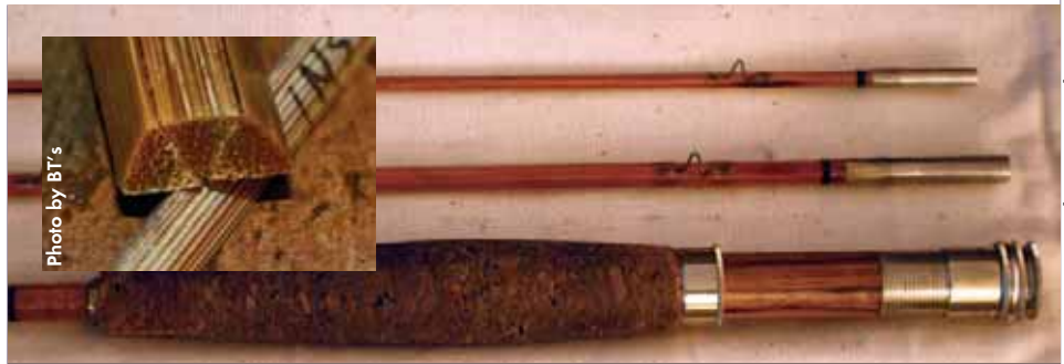
The prepared bamboo pieces are triangular in shape, with two sides coming from inside the bamboo culm and one from the outside. Here, the half-round illustration prepared by the author has the center piece installed with one of the "in" sides facing out – a mistake.
