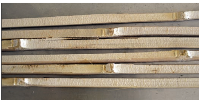
Strips laid in a 3x3 stagger ...
