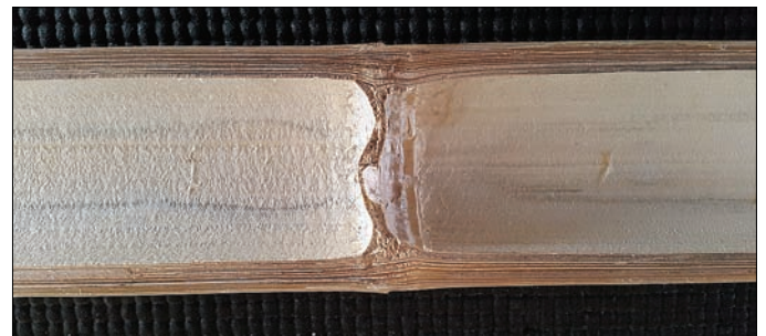
Nodal dams are visible after splitting the bamboo culm.
