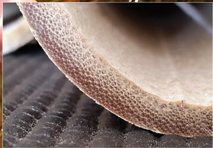
Side view of a bamboo culm showing the dense power fibres just below the enamel.
