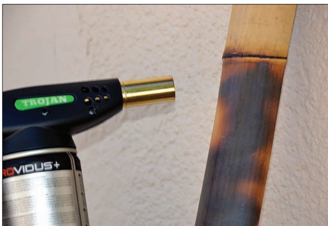
Flaming the bamboo culm with a propane torch.
