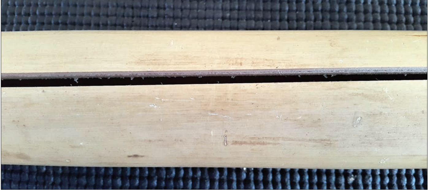
All bamboo culms should have a drying split that runs the entire length of the culm.
