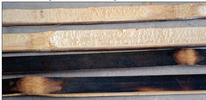
Strips showing flattened nodes on both pith and enamel sides.
