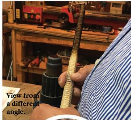
A close up to show the difference between the unflamed and flamed part.
