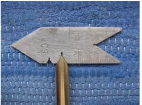
You can also use a square piece of steel or brass, or a hexagonal one, and turn it round after having ground the 60°- wedge-tip.
