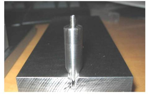
A wedge-tip with threads to screw to the shaft of the dial indicator.
