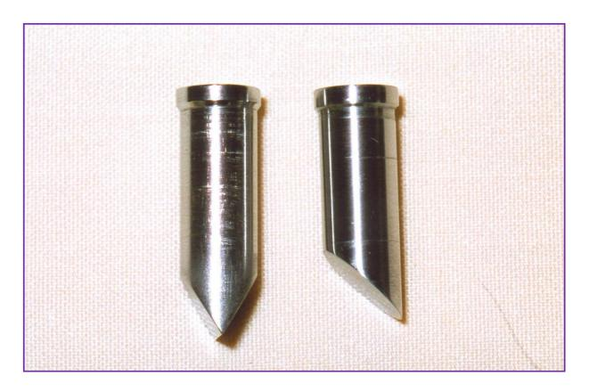
I have also made a contact point and a corresponding calibration tool for my quad-forms, which works just as well. Planing-forms and calibration devices for a five sided rod I do not have, though. But I have included the necessary information to make one.
