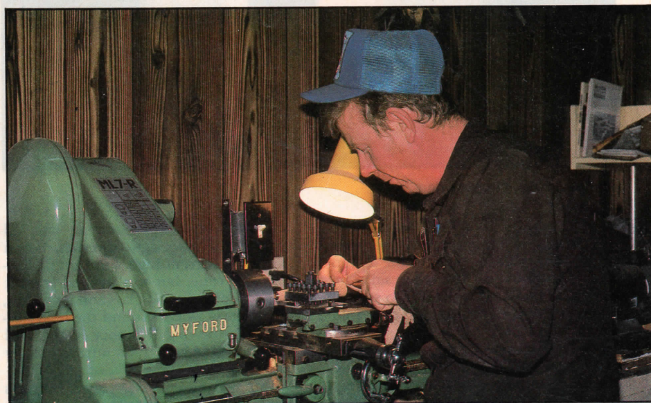
Andersen shaping and smoothing handle and reel seat in the lathe.
