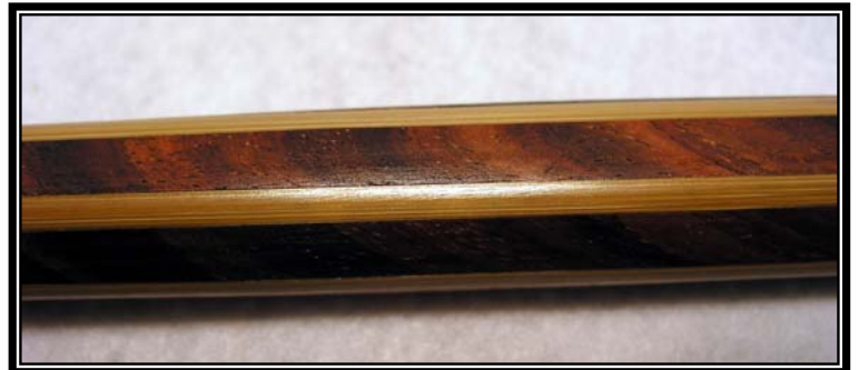
The rod will have no cork and thus the shaft is the grip itself which makes the rod slightly slicker when fishing but it also makes it much more responsive due to the lack of the insulating and dampening features of cork. Above right is the rod after glue up and sanding and several coats of hand rubbed finish.
