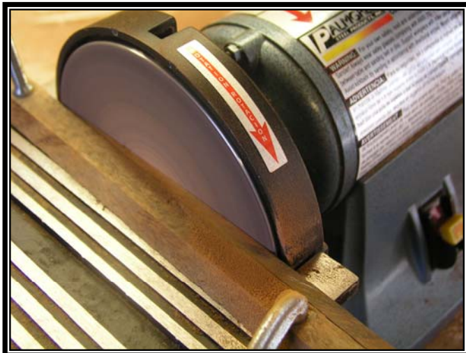
Strip being sanded on the disc sander. Strips tapered on the disc sander and ready to be feathered.
