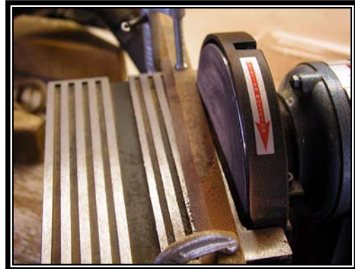
Strips center marked; top and bottom with one tapered. The fence on the disc sander.
