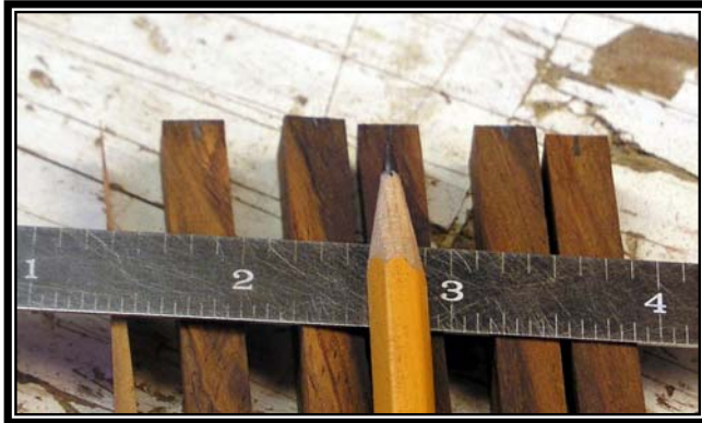
Strips center marked; top and bottom with one tapered. The fence on the disc sander.
