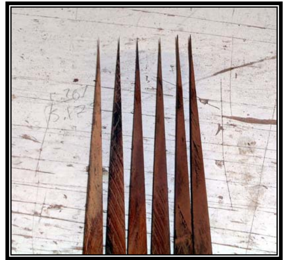
Strip being sanded on the disc sander. Strips tapered on the disc sander and ready to be feathered.
