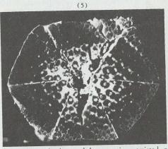
Photo 6 shows a spinning rod butt section, twisted one complete turn in 5 inches. This is the most severe test we could think up. This specimen shows absolutely no failure of glue seams under a powerful glass. Two panels of cane split just a trifle on opposite sides, but the section returned to its original straight condition, and would still do a very good job if put into a rod. This is on display in our shop.
