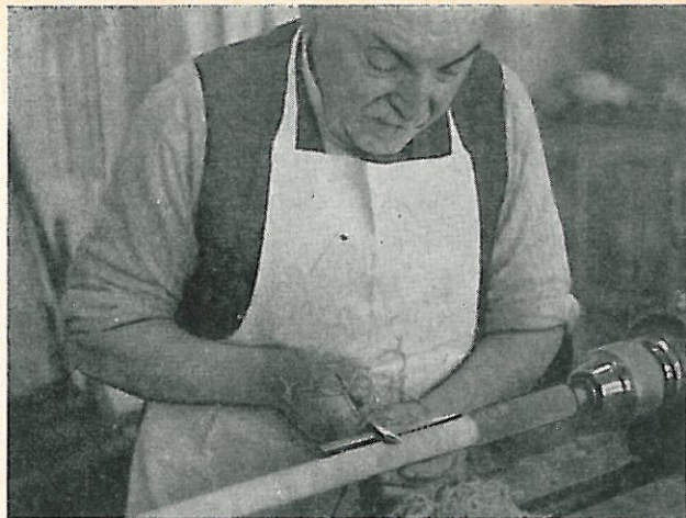
One of our old craftsmen turning the cork handle of a rod
