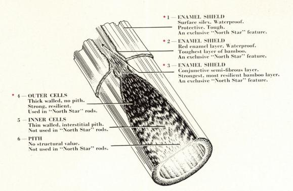
★ Only the strongest and toughest layers of bamboo are used in "North Star" rods. Expertly fitted to within .001" of theoretical perfection, in accordance with scientific rod action charts, "North Star" rods feature EVENLY BALANCED FLEXIBILITY, DYNAMIC FLASH-LIKE ACTION, EXCEPTIONAL POWER and THRILLING CASTING ACTION.
