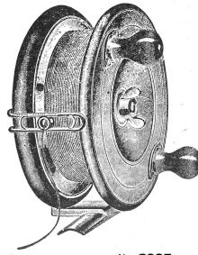
solid mahogany, beautifully finished, brass bound throughout, s o that it cannot be affected by climatic conditions. Of center pin construction, it is very easy running. Tool steel pinion, heat treated and hardened, run in by hand on hard brass bearing. Patent line guard. Steel gear and pawl. Very heavy click spring. Substantial handle of polished hardwood. Click optional
