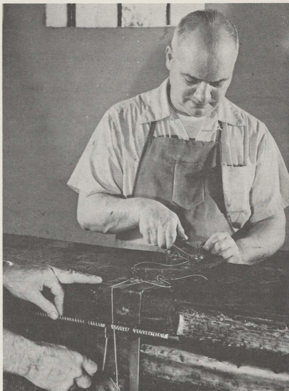
and then cross wrapped under tension to form a hexagonal section in which the seams are visible. (C) Oven heat is used to "set" the cement. After cleaning, the sections are
