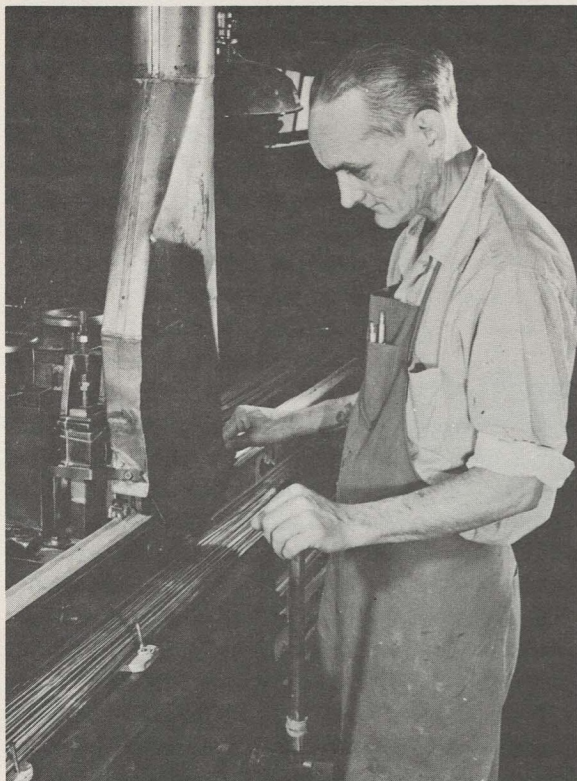
Three steps in rod making. (A) The specially designed milling machine mills segments as light as 3/100 of an ounce. (B) Six milled segments are immersed in Bakelite cement,
