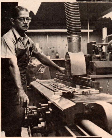
Morris Pennock at the milling machine, turning our bamboo segments to an accuracy of one-quarter of a thousandth of an inch.
