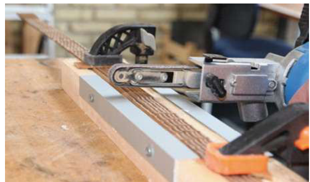
Device to Control Depth of Sanding when Hollow Building.
